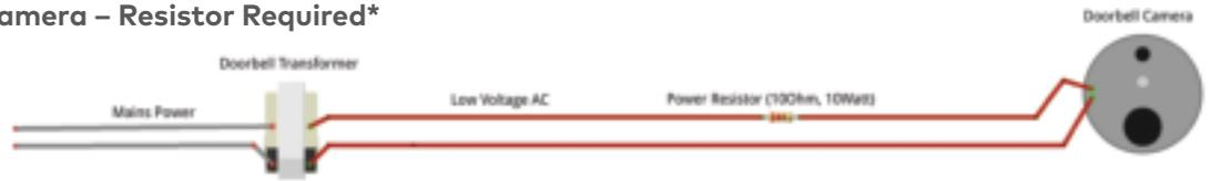
**WARNING:** This setup is designed for testing and demonstration purposes only. Failure to install a resistor (10 Ohm, 10 Watt) when a chime is not present may result in damage to the doorbell camera.
