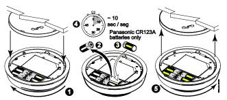
CAUTION: The batteries used in this device may present a fire or chemical burn hazard if mistreated. Do not recharge, disassemble, heat above 100°C (212°F) or dispose of in fire. Use only Panasonic CR123A Lithium batteries. Use of other batteries may present a risk of fire or explosion. Keep used batteries away from children. Dispose of used batteries properly.
